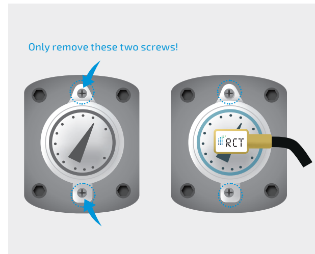
Fig. 2+3 | Removing original dial and installing RCT sensor
